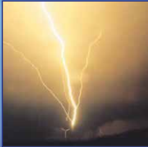
Real Lightning Test Performed by Triggering Lightning with a Rocket
