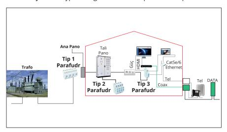
lightning strikes, Type 2 surge arresters are preferred in panels that may be affected by indirect lightning strikes or switching, and Type 3 surge arresters are preferred in device feeds.
