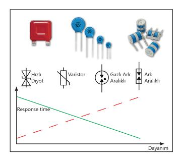
An A.G. surge arrester contains at least one non-linear component. The electrical resistance of this component varies depending on the voltage applied to it. Four types of components are typically used in the Radsan surge arrester group. Since each component has different advantages and disadvantages, combined-hybrid surge arresters have been developed by combining the advantages of both technologies to achieve the best results.
