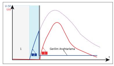
These are switching-class low-voltage surge arresters, designed to protect against high-amplitude surges and operating using the spark gap principle. They can easily withstand strong surges, but due to their somewhat long response times, they cannot protect against low-amplitude, weak surges. They are designed for the first stage of overvoltage protection.
