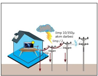
When lightning strikes the lines surrounding the structure and supplying it, the lightning current flows through the line to the structure and causes excessive voltage.
