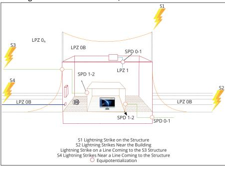
LPZ O<sub>A</sub>: This is an open area not protected by an external lightning protection system. Equipment in this area must be exposed to direct lightning strikes and withstand all lightning current and magnetic field effects.
