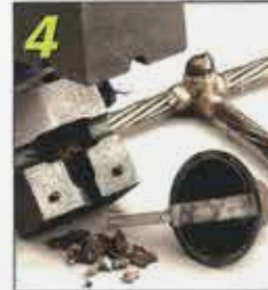
4 Open the mould and remove the expanded steel cup – no special disposal required
